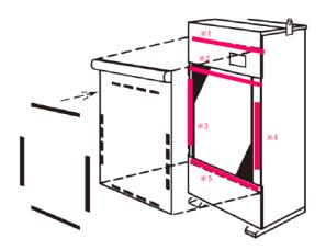
Daikin's roll filters are easy install and requires little maintenance. Rolls comes with magnets on the back which sticks to your chiller. Just roll down the filter and snap in place. When its time to change, simply cut away the used roll and roll down a new section.
